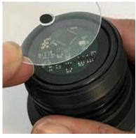
Place the disc on top of the probe body with the green spot against the body. Do not touch the spot on any side with your fingers.
