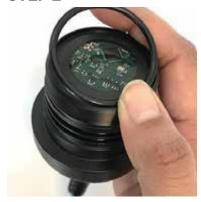
Place the O-ring in the recess on the top of the probe body.
