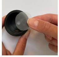
Place the reinforcement grid inside the probe cap.
