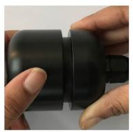
Screw the probe cap and body carefully together.
