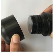
The disc is centered on top of the probe body. Put the probe cap over the disc.
