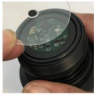
Place the disc on top of the probe body with the green spot facing down (the blackup). Do not touch the spot on any side with your fingers.
