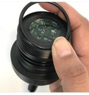
Place the O-ring in the recess on the top of the probe body.
